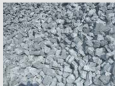
Coke manufactured by carbonizing metallurgical coal
