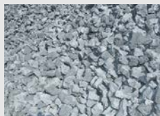
Coke manufactured by carbonizing metallurgical coal
