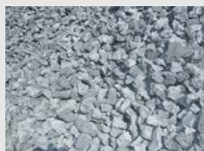
Coke manufactured by carbonizing metallurgical coal
