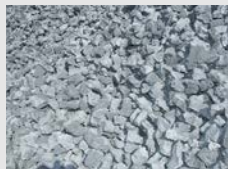
Coke manufactured by carbonizing metallurgical coal
